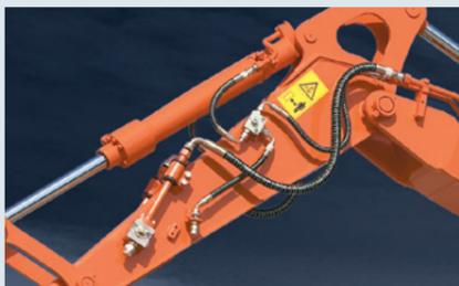
**Front oil leakage preventing valve**
