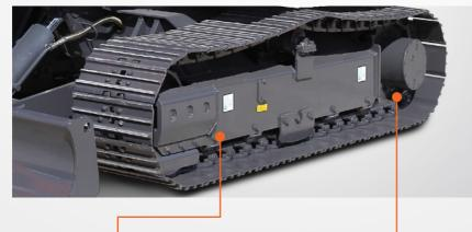
The track roller attachment point was shifted from lower to middle portion to improve undercarriage stability and structural rigidity of the chassis.
