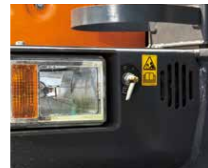
BATTERY ON-OFF SWITCH
