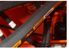
High quality hydraulic hose Parker hoses are applied for all high pressure hydraulic line to improve piping quality
